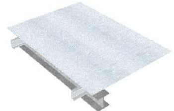
Step 2 -Laying out Aluminium Foil for vapour and radiant control.
